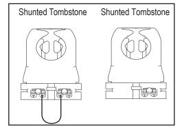
Note: Tombstone wiring should have one side Hot (L) and other side Neutral (N). Tombstones may vary based on what is currently installed in the fixture.
